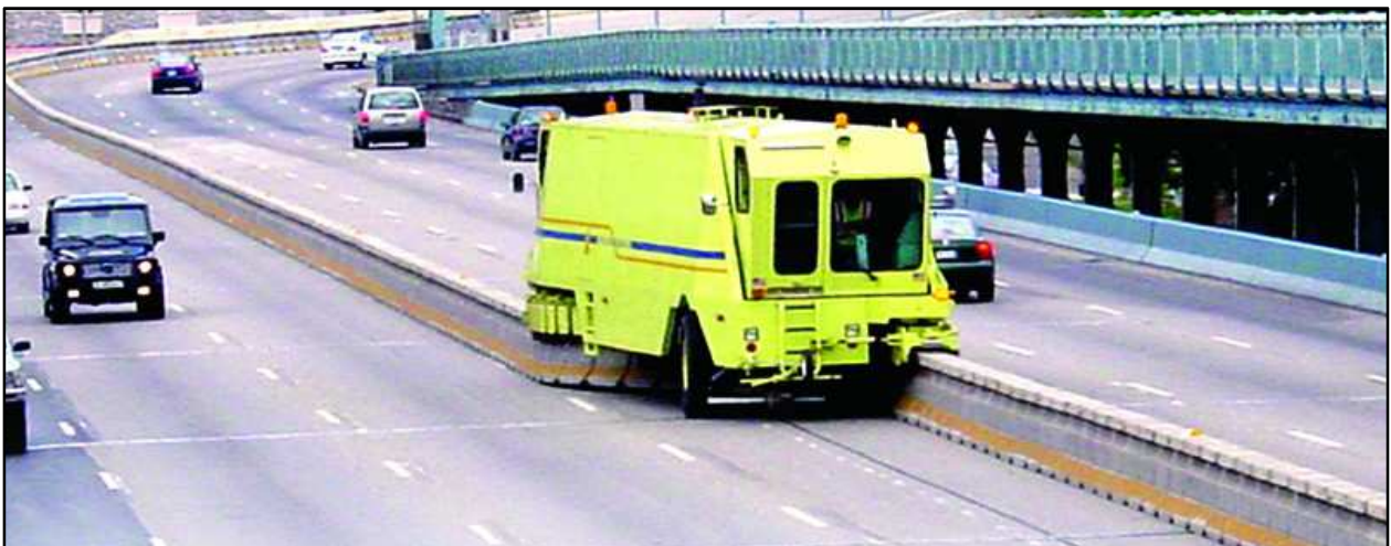
Figure 6: Moveable barrier system in operation
